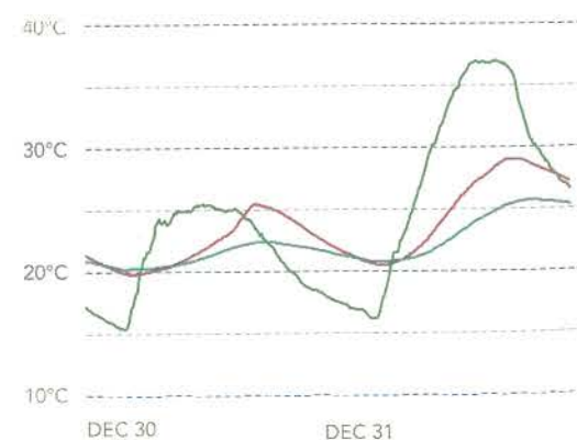
Temperature monitoring graphs show one apartment's performance without air-conditioning assistance. Kitchen sill temperature shows heat transfer through aluminium window frames. Timber frames were specified in the design but aluminium were subsequently installed by the developer.
