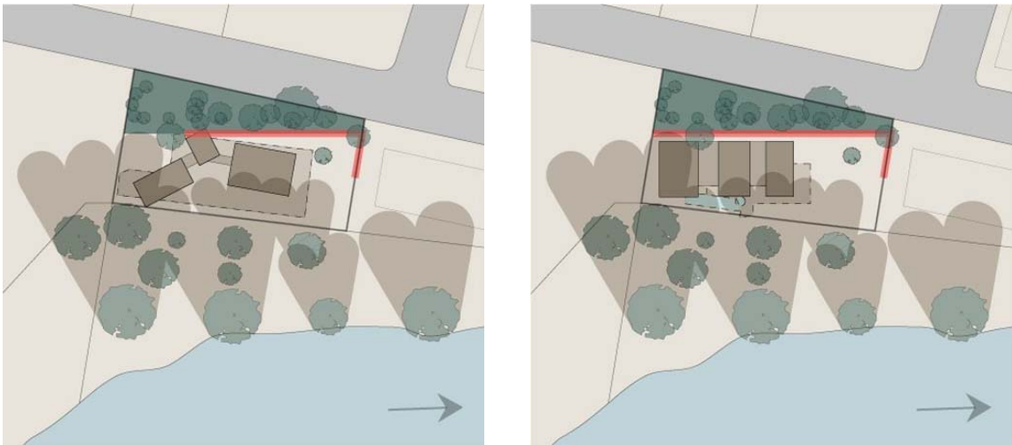
Figure 8 & 9 Diagrams of early design and final design showing shadows cast by trees and courtyard wall
